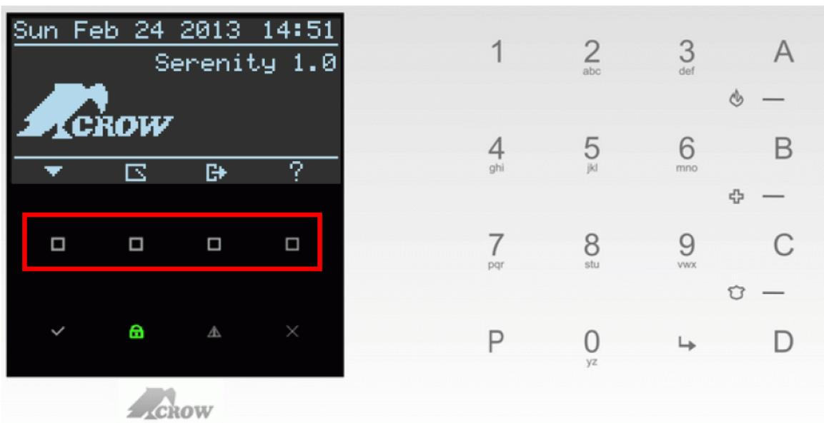
**Important Note:** Multiple programming function touch buttons (above marked in red) change functionality according to menu level. Functionalities are displayed on status symbols display area.
