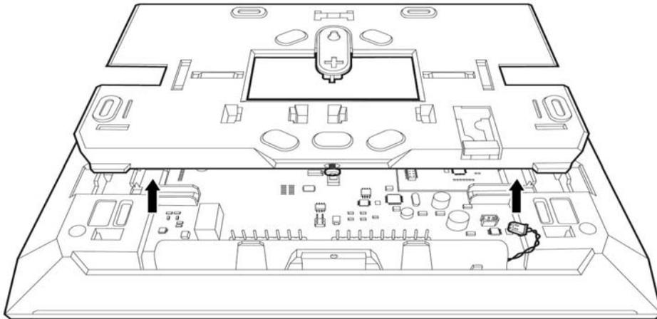
Connect wires into terminal blocks according configuration requirements (see "Connection Diagram") and screw the bracket on the wall.
