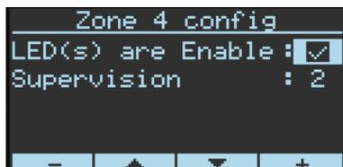
**Important Notice:** 1. Setting or changing of Zone Configuration will be implemented into the detector configuration in the next event such as Open Zone \Open Tamper \ supervision.
