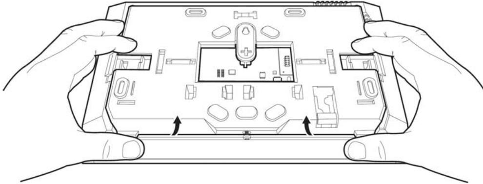
Remove the bracket from the panel
