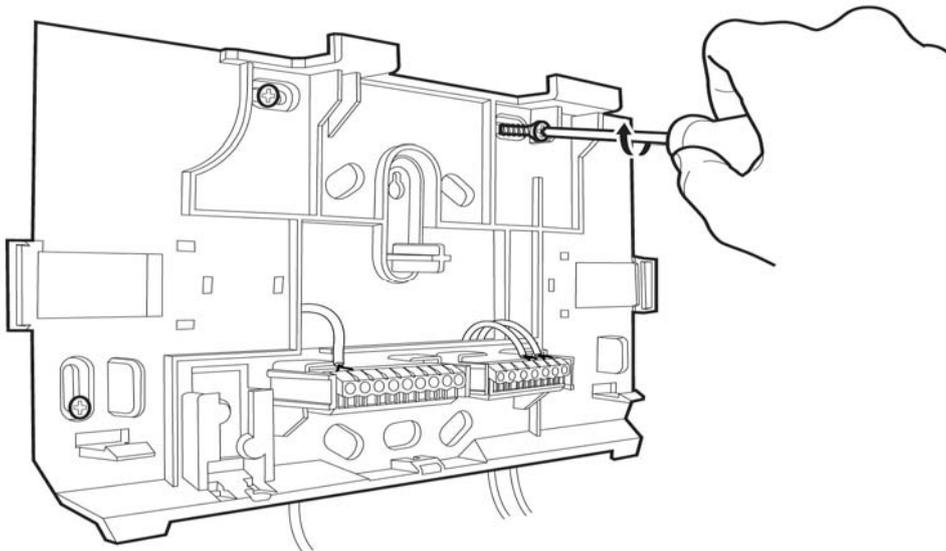
Once all connections are made, connect the battery and mount the panel on its bracket.
