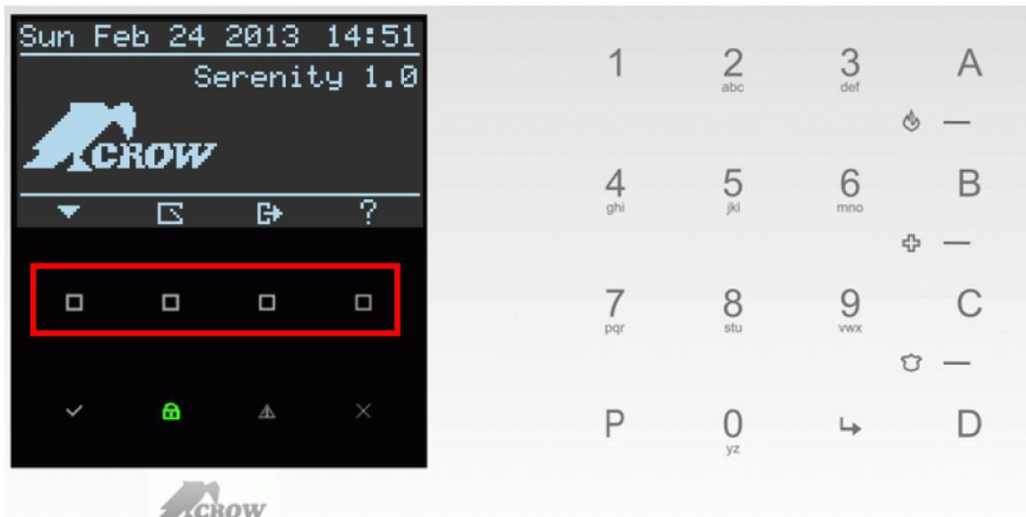
**Important Note:** Multiple programming function touch buttons (above marked in red) change functionality according to menu level. Functionalities are displayed on status symbols display area.
