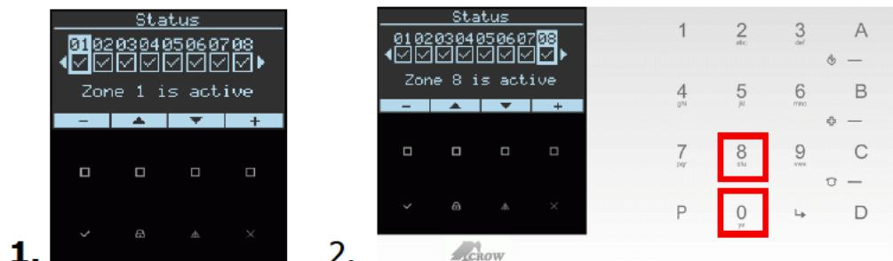
Option 1: Installer can use the buttons " + or - " to move between zone numbers
