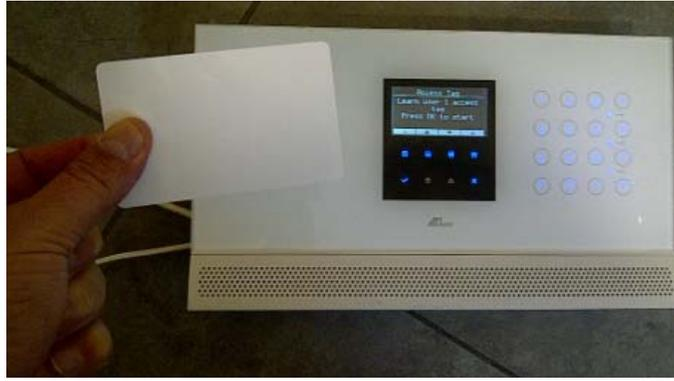
The Serenity's RFID reader is used for selective arming or disarming Area 1,3,2,4 or all. In addition it can be used to perform actions, for instance, to turn on/off an output.
